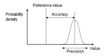
Due to non-random or systematic errors, the readings or measurements may be *precise* but *not* accurate e.g. measuring the mass as 21.3456 kg when it is 50 kg. This may be due to a wrong setting on the instrument, using the wrong formula or equation or the observer not being able to clearly see the dial.
